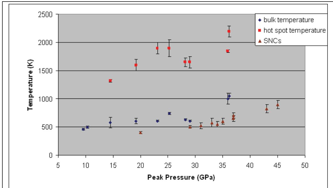
**Fig. 1.** Pyrometry results compared to SNC meteorites [9]. Bulk temperatures over typical range of meteoritic shock pressures show modest increase after shock, while hot spot temperatures reach melting.
