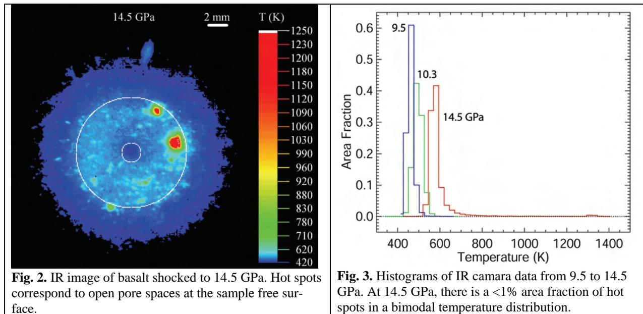
**Fig. 2.** IR image of basalt shocked to 14.5 GPa. Hot spots correspond to open pore spaces at the sample free surface.
