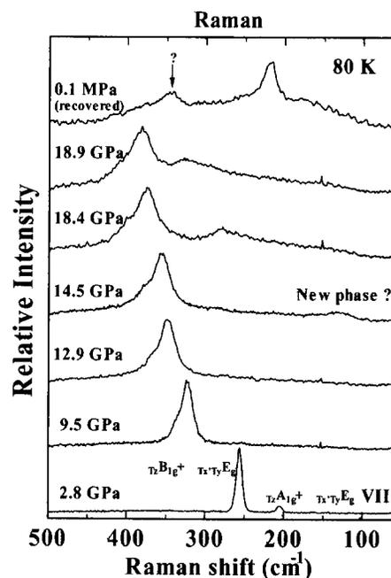
FIG. 6. *In situ* Raman spectral changes of ice VIII at 80 K in the region of the rotational and translational vibrations (50–500 cm<sup>-1</sup>) as a function of pressure.
