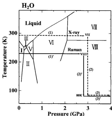
FIG. 1. Schematic experimental paths (1)–(3) and (1)′–(3)′ performed in the present study on the equilibrium phase diagram of H<sub>2</sub>O. (...) Paths for the x-ray measurements. (—) Paths for the Raman measurements.
