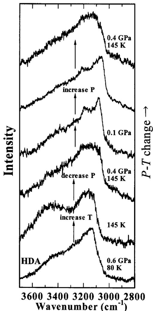
FIG. 3. HDA probed by *in situ* Raman OH stretching spectra as functions of pressure and temperature.
