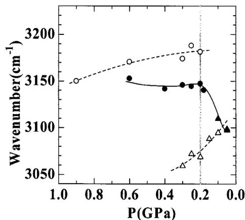
FIG. 6. Comparison of Raman frequency changes between Figs. 3 and 5 upon decompression: HDA ( $\circ$ ) and LDA ( $\triangle$ ) in Fig. 5, and the corresponding peaks ( $\bullet$ ) and ( $\blacktriangle$ ) in Fig. 3. The vertical thick line shows the estimated transition point between the two phases. The solid and dashed curves are guides to the eye.
