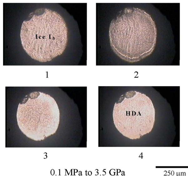
FIG. 2. (Color online) Photomicrographs showing the transformation of ice I<sub>h</sub> to HDA from near 0.1 MPa to  $\sim 3.5$  GPa. The gray areas in images 2 and 3 show the mixed phase parts of the sample during the course of the transition.
