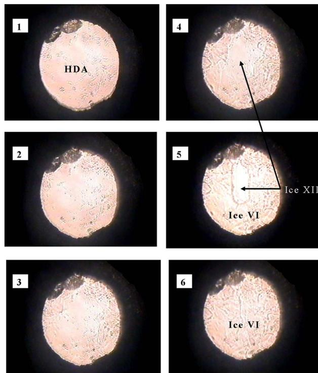
FIG. 8. (Color online) Photomicrographs showing the transition from HDA to ice XII, then finally to ice VI. The  $P$ - $T$  conditions were  $\sim 1.25$  GPa and 158–168 K, and the time evolution is about 15 min. Ice XII is the clear rectangle portion of images 4 and 5. Upon further heating complete crystallization to ice VI occurred, as shown in image 6.
