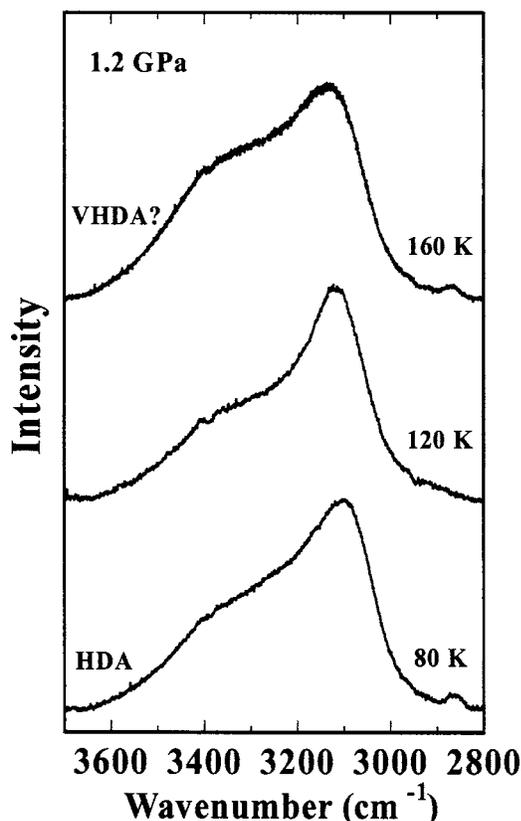
FIG. 7. HDA probed by *in situ* Raman spectroscopy in the region of the OH stretching bands as a function of temperature near  $\sim 1.2$  GPa (path 3').
