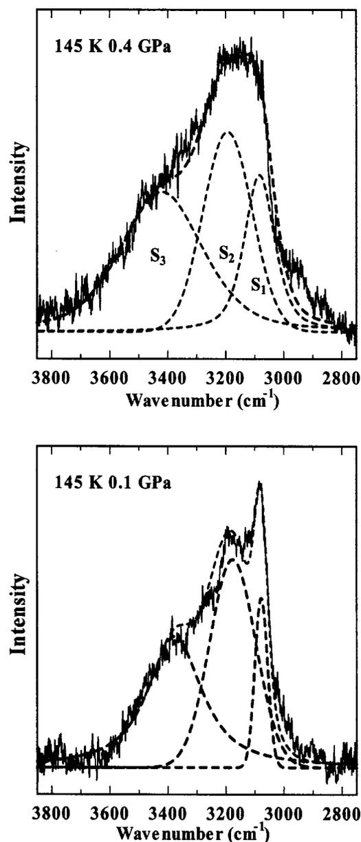
FIG. 4. Representative band component analyses of Raman OH stretching bands following the pressure-induced reversible transition between the two phases at  $\sim 145$  K. Dotted lines represent deconvoluted peaks.
