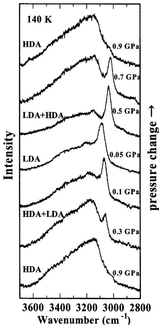
FIG. 5. *In situ* Raman spectra in the OH stretching region measured during the pressure-induced reversible transition between LDA and HDA at  $\sim 140$  K (path 4'). We prepared the LDA and/or HDA samples by methods described in the literature. (Refs. 29 and 31). HDA transformed to LDA completely at  $\sim 0.1$  GPa, whereas the LDA changed to HDA at 0.8–0.9 GPa in our measurements.
