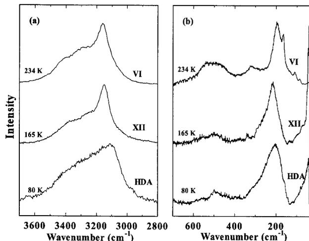
FIG. 9. *In situ* Raman spectra following the transition from ice  $I_h$  to HDA and ice XII as a function of temperature at  $\sim 1.2$  GPa. (a) OH stretching region; (b) low frequency lattice vibration region.
