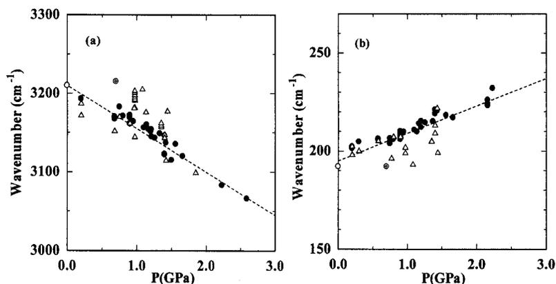
FIG. 10. Pressure dependences of the (a) OH stretching and (b) low frequency lattice mode frequencies at various temperatures.  $\bullet$ : ice XII,  $\Delta$ : ice VI,  $\circ$ : phase reported by Chou *et al.* (Ref. 24),  $\circ$ : ice XII from Salzmann *et al.* (Ref. 25). The dotted line is a least-square fit of our ice XII data.
