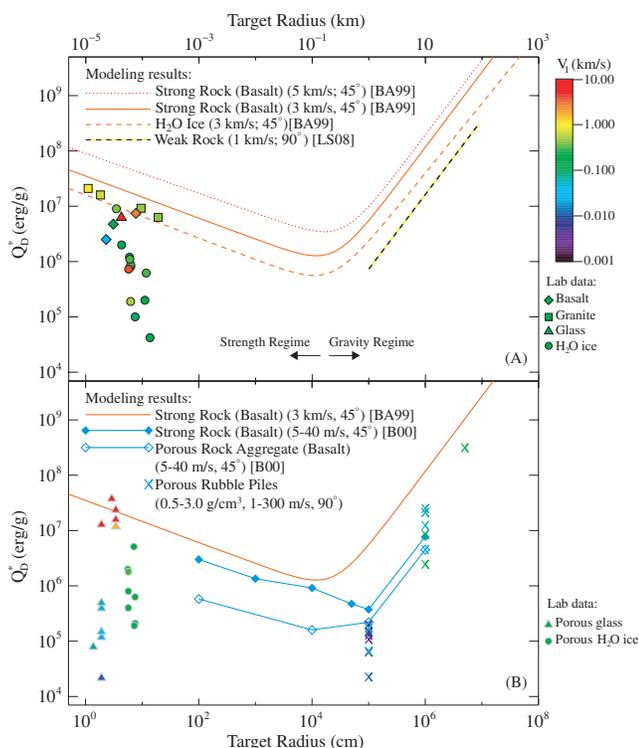
**Figure 1.** Traditional catastrophic disruption criteria ( $Q_D^*$ ) as a function of target radius. Color denotes impact velocity. (A) Nonporous materials: numerical (Benz & Asphaug 1999; Leinhardt & Stewart 2009) and laboratory experiments (see the text). (B) Porous materials: laboratory data on glass and ice (see the text) and numerical experiments on aggregate rock (Benz 2000) and rubble piles (this work). High- and low-velocity  $Q_D^*$  for nonporous basalt are shown for reference.
