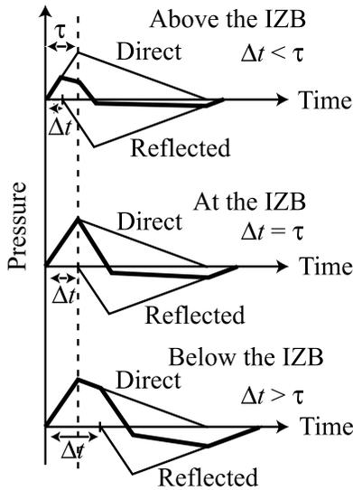
**Figure 1.** Schematic of interaction between triangular-shaped direct and reflected waves above, at, and below the interference zone boundary (IZB) [after Melosh, 1984]. The pressure history of the material is the sum of the two waves (thick solid line).
