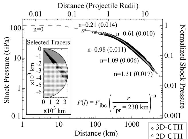
**Figure 2.** Shock pressure versus radial distance from a burial depth of  $0.7 \cdot r_{\text{pr}}$  recorded by tracers below the interference zone in the crust and upper mantle (inset), for a 230-km radius projectile at 9 km/s. The 2D (triangles) and 3D (diamonds) results are nearly identical. Power-law exponents are indicated with standard deviations in parentheses.
